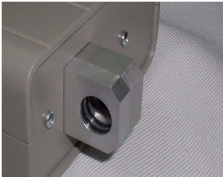
FIGURE 2-2 Aluminum Block with Microphone Ports
