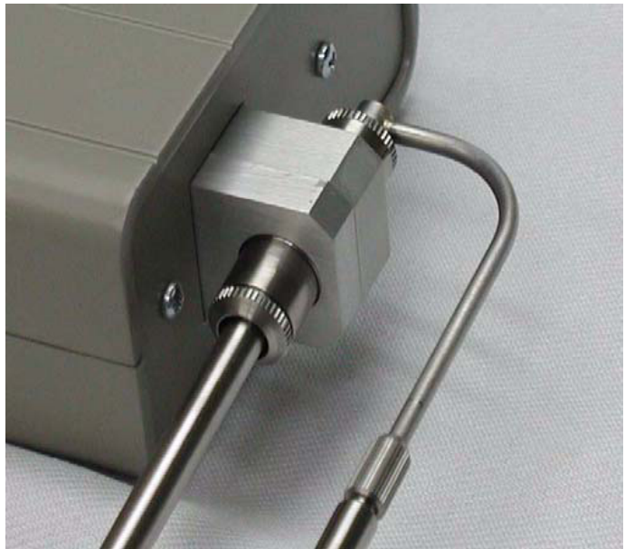
FIGURE 3-1 Microphone In Place Inside Microphone Ports of CAL291
